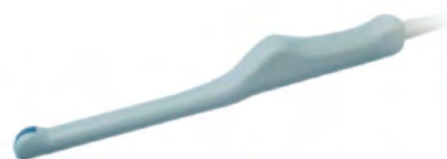
Microconvex endowaginalna: CV-580 / R13 (5,0~10,0 MHz)
